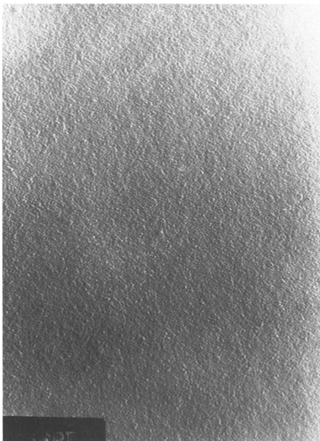
Fig. 8. TEM replica picture from the thinned sample given by curves b in figs. 1 and 2. Magnification is 75000.
